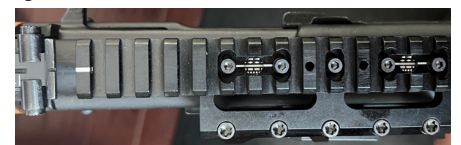
Fig. 4b: Example of alternative correct Picatinny Rail alignment with the rear iron sight
