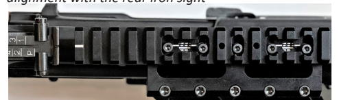
Fig. 4b: Example of alternative correct Picatinny Rail alignment with the rear iron sight
